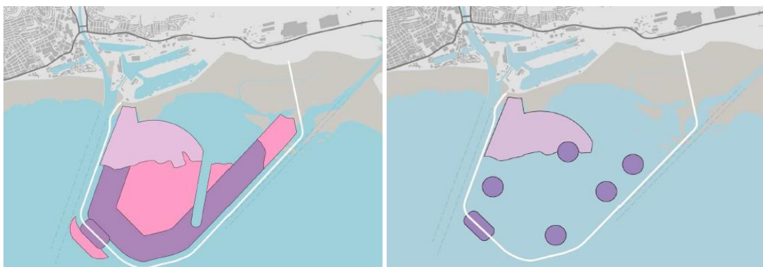
Figure 3 Dredging options from the Applicant's ES: An extensive, shallow option and a less extensive, deeper option.
